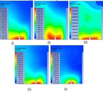
**Fig. 5:** Contours of pollutant mass fraction on (i) Plane A1A2, (ii) Plane B1B2, (iii) Plane C1C2, (iv) Plane D1D2, and (v) Plane E1E2
