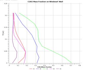
Fig.9 (ii): Pollutant mass fraction plots along sample lines on windward side.
